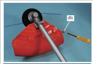
1. Remove shield piece (A) by removing screw (B), and expand nylon lines, and cut nylon lines to 225 mm for proper engine loading to adjust carburettor correctly.
