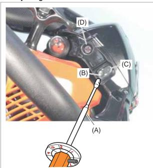
1. Start and warm engine for 100 seconds alternating engine speed between WOT 5 seconds and idle 5 seconds. Turn H mixture needle (C) anticlockwise until engine speed drops to approx. 12,000 r/min at WOT.
