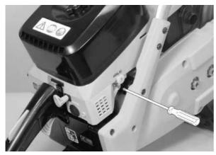
2. Screw 2.5 mm wood screw into the center of the L limiter cap.
