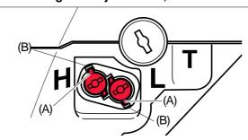
1. Turn L and H mixture needles out anticlockwise to rich stop, and meet limiter cap tab (A) with locating slot (B).
