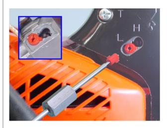
4. Screw thread of limiter cap tool 91019 into other centre hole of the other limiter cap anticlockwise until the limiter cap is pulled out from the mixture needle completely. Remove the limiter cap from limiter cap tool turning clockwise, and screw thread of limiter cap tool 91019 into centre hole of previous limiter cap to pull out completely.
