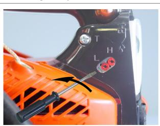
1. Turn the L and H mixture needles out anticlockwise until side of rich stop to meet limiter cap tab (A) with locating slot (B), using 2.5 mm blade screw driver.
