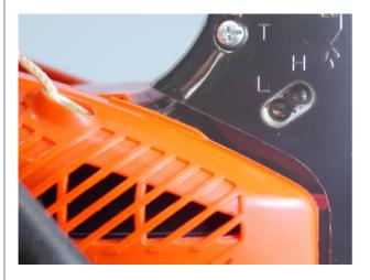
5. Turn L and H mixture needle clockwise until lightly seated, and then turn out both needles following turns.
